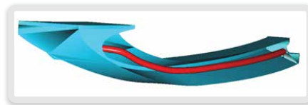
Figure 1. LED light guide daytime running light (DRL) feasibility study with luminance visualization in XYZ color rendition of the light
